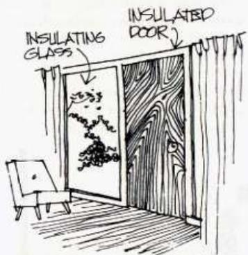
**Figure II-C-15.** Provide the advantages of a sliding glass door without much of the energy waste by using a fixed pane of insulating glass and an insulated door.
