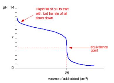
4- The third curve shows a weak acid being titrated by a weak base This is the reaction of ethanoic acid vs ammonia. As you can guess, the steepest point in the curve is now harder to identify since the pH is not changing as rapidly. Of course, we can graph the derivative of the curve for more accurate determination. However, we can't simply just look at the curve to point out the equivalence point as before.
