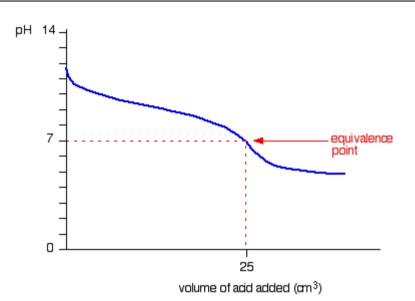
Another way you probably learn to perform a titration is not to track its pH but to use an indicator. We know the endpoint is defined as when the solution changes color (like colorless to pink). A problem with weak acid/weak base titration is the lack of available indicator to accurately determine its end point.
