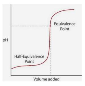
The second point is the higher equivalence point. Once the acid has been neutralized, notice the point is above pH=7. When a weak acid is neutralized, the solution that remains is basic because of the acid's conjugate base remains in solution.
