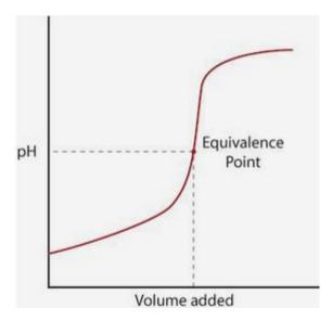
2- The second curve shows a weak acid being titrated by a strong base
